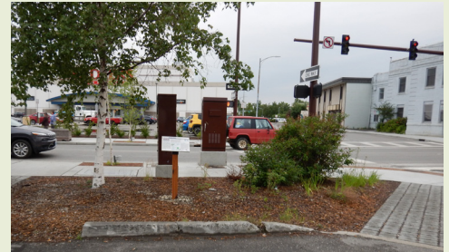
Transit Park is using green infrastructure such as stormwater trees and permeable pavers to help retain rainwater and soak it into the ground. Photo Credit: Alaska DOF.
